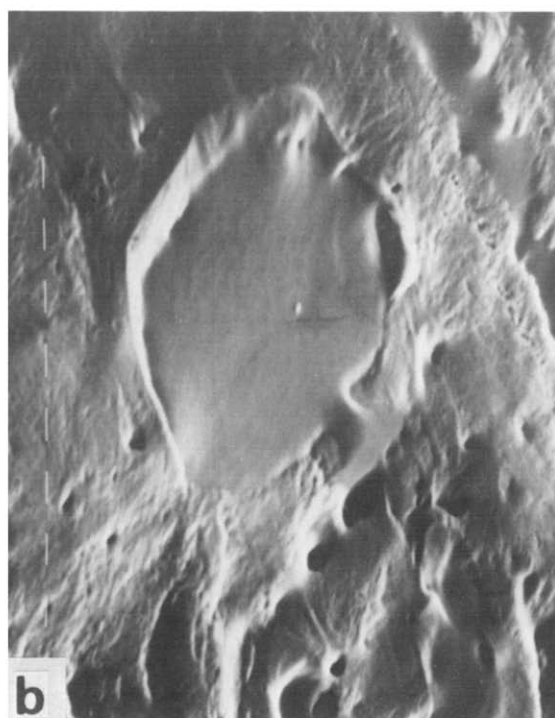
Figure 4 SEM micrographs of a microtomed surface of ternary blend B (80/10/10): (a) low magnification ( 640\times ); (b) high magnification ( 5000\times )
